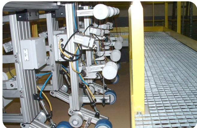
The PRS350 is a custom built, semi automatic system for applying Rippatape® to carton packaging. Sited between the rotary sheer and slitter scorer, the integrated design comprises a platform and multiple application heads. The system is ideally suited to high volume users of Rippatape®.
